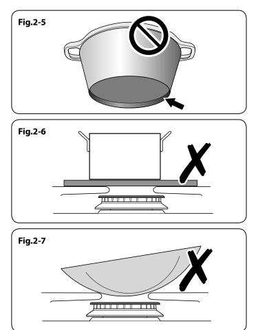
Pans and kettles with concave bases or down turned base rims should not be used (Fig.2-5).
